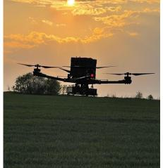
storage box that can adjust the temperature of cargo. These drones can deliver the necessary medicines to hot spots in Ukraine and occupied cities that are inaccessible.
