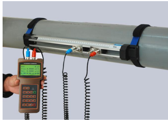
OI-TUF-2000H Type Handheld Ultrasonic Flowmeter
