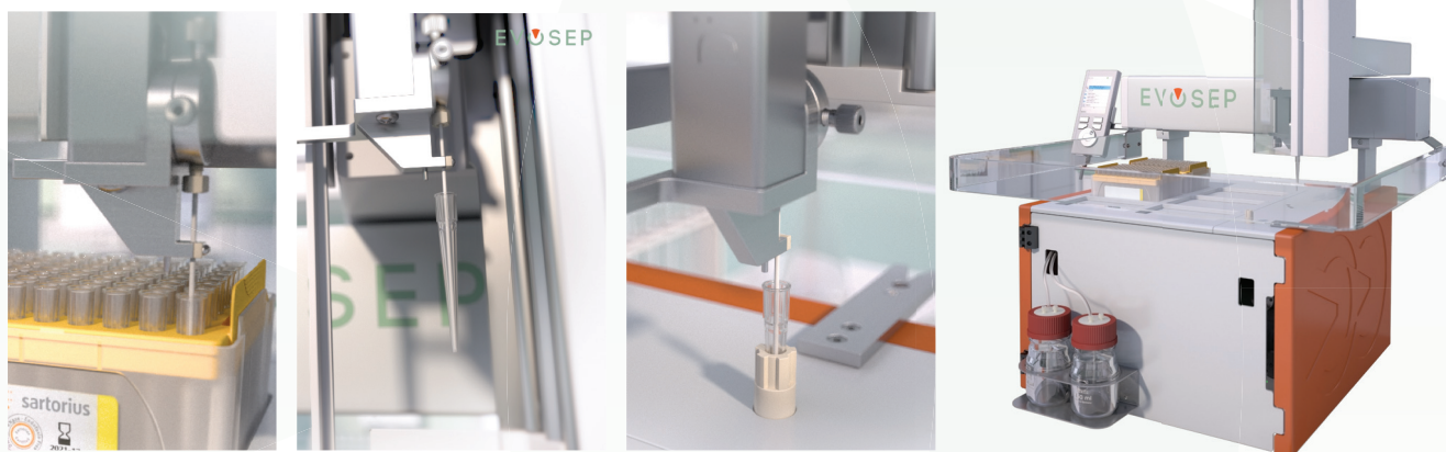
Figure 1: Evosep One and a close-up of the pipette tip-based sample handling
