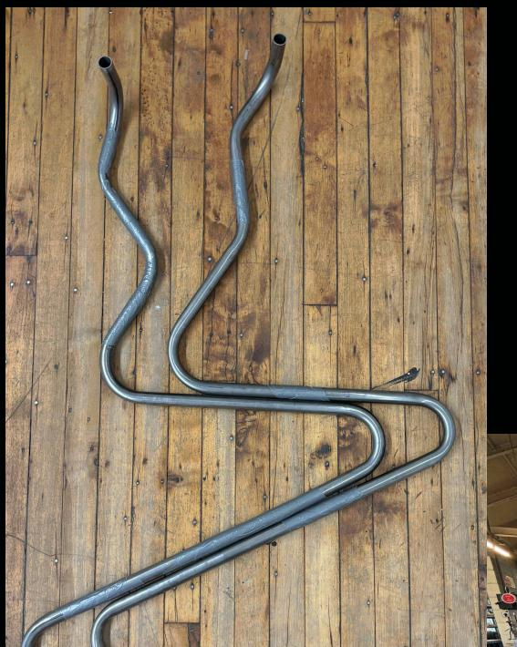
Using 1" OD steel tubing and a Hossfeld bender, I shaped mirrored side frames. Every curve was refined through physical iteration, learning and adjusting at every step. The breakthrough came with the backrest sling, laced like a corset, it introduced tension, transforming the project into a tool free assembly.
