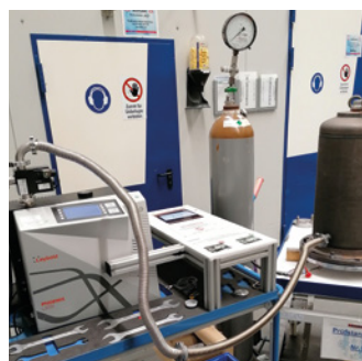
3d Helium, Fugitive Emission Test (FET) Option code F28 / F29
