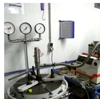
4b Helium, Leakage detection in vacuum Option code M86
