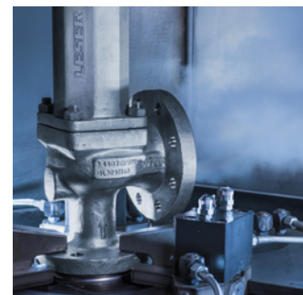
4c Helium seat tightness test under cryogenic conditions Option code M80
