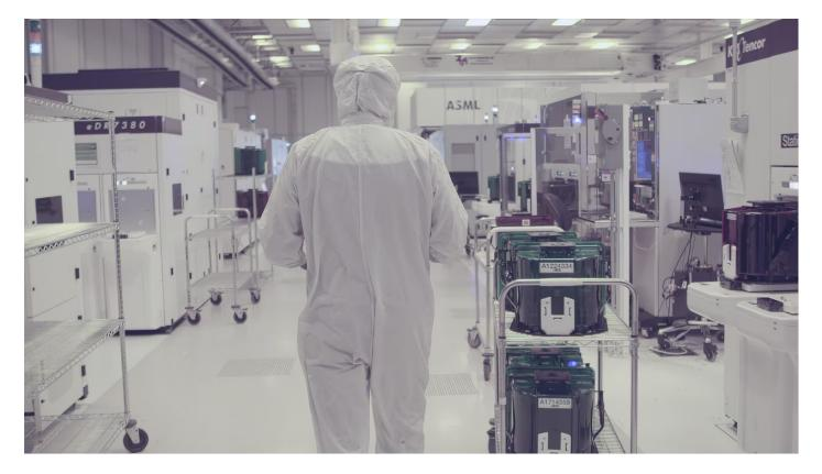
A worker walks through the Albany NanoTech Complex clean room. In the background is an extreme ultraviolet lithography (EUV) machine made by ASML, a Dutch company that is the sole manufacturer of EUVs. Micron Technology plans to use EUVs in its semiconductor fabrication plants in Clay.
