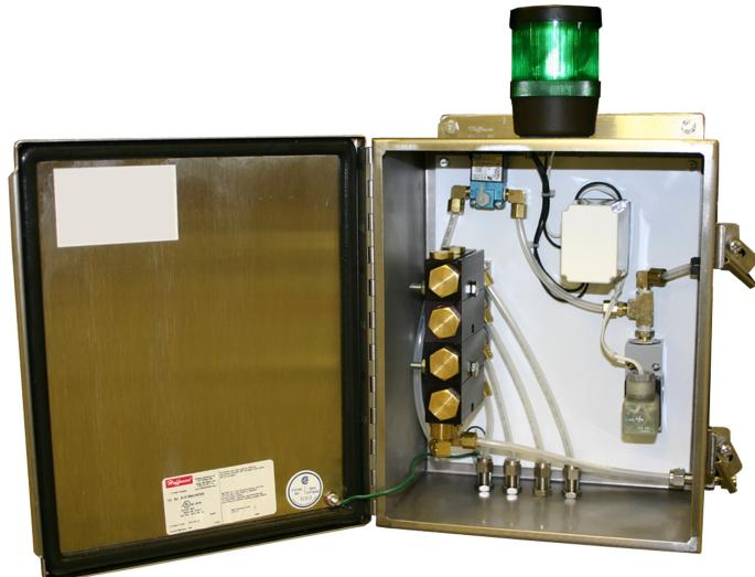
**System includes:** Logic control cabinet with indication light, stand, pumps (3), timer, air pressure sensor, solenoid valve, tubing and fittings. Lubricant is pulled from a 55-gallon drum.
