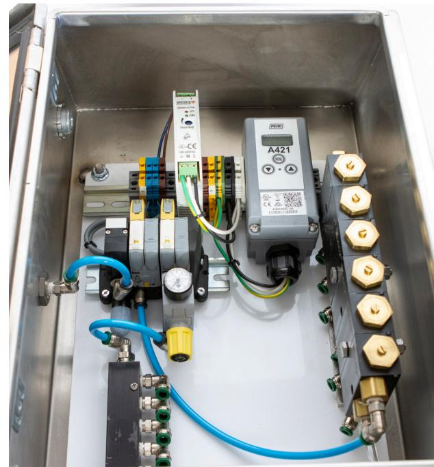
Most connections are "push" style for ease of removal / installation.
