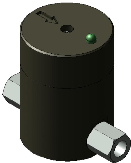
Simple solutions for grease flow verification by GOLD. Opaque grease lines do not allow for visual inspection of lubrication system output. Oval gear flowmeters serve well to indicate grease flow in lubrication systems. To eliminate the need for a PLC or HMI, GOLD has developed this simple, self-contained, flashing flow detection device.
