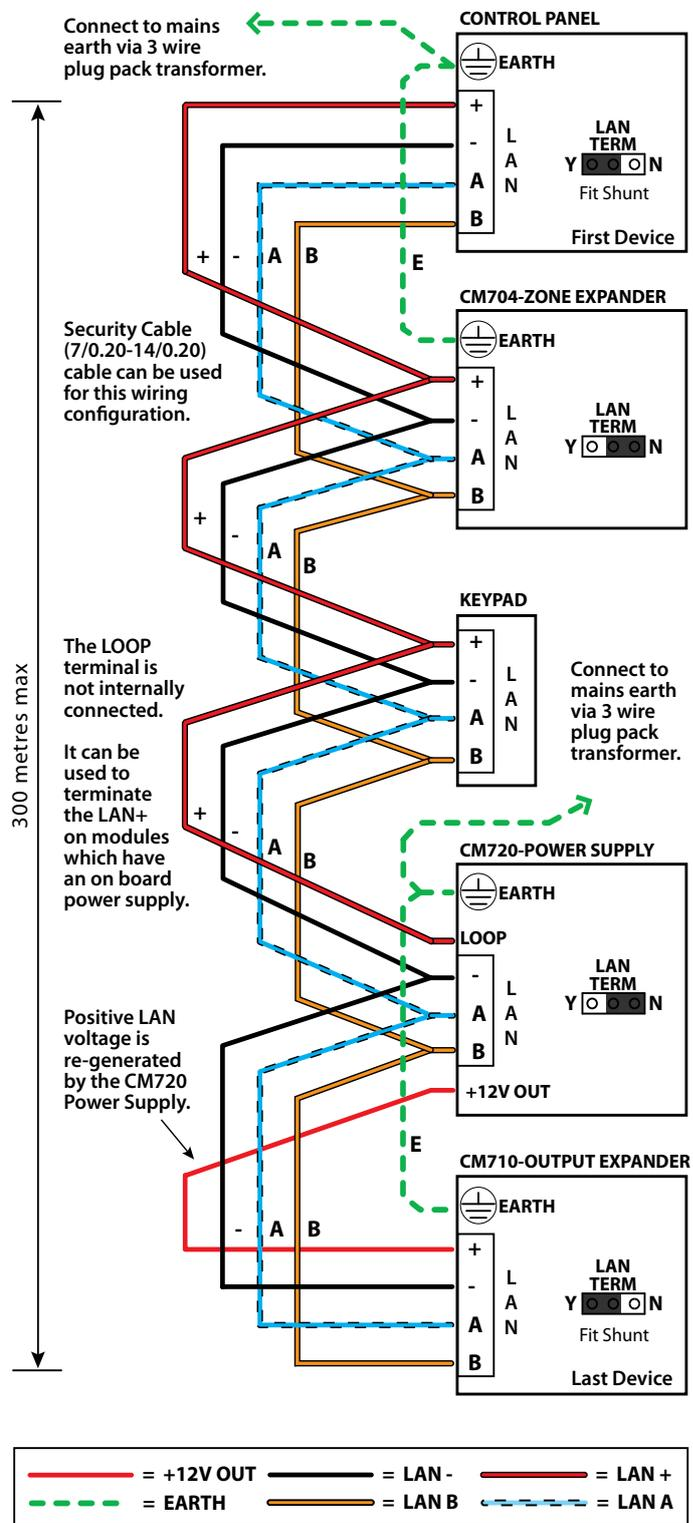
**Figure 18: LAN Connection Using 2 Pair Security Cable**
