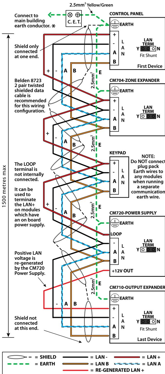
Figure 19: LAN Connection Using Twisted Pair Cable
