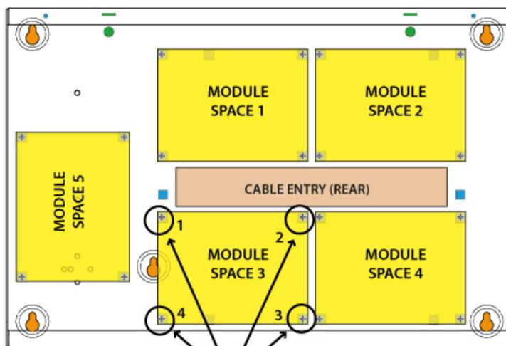
When installing small modules, you should fit 4 mounting clips as shown.
