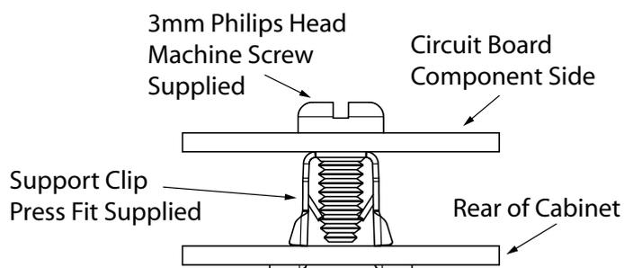
**Figure 1: PCB and Mounting Clip Installation Diagram**
