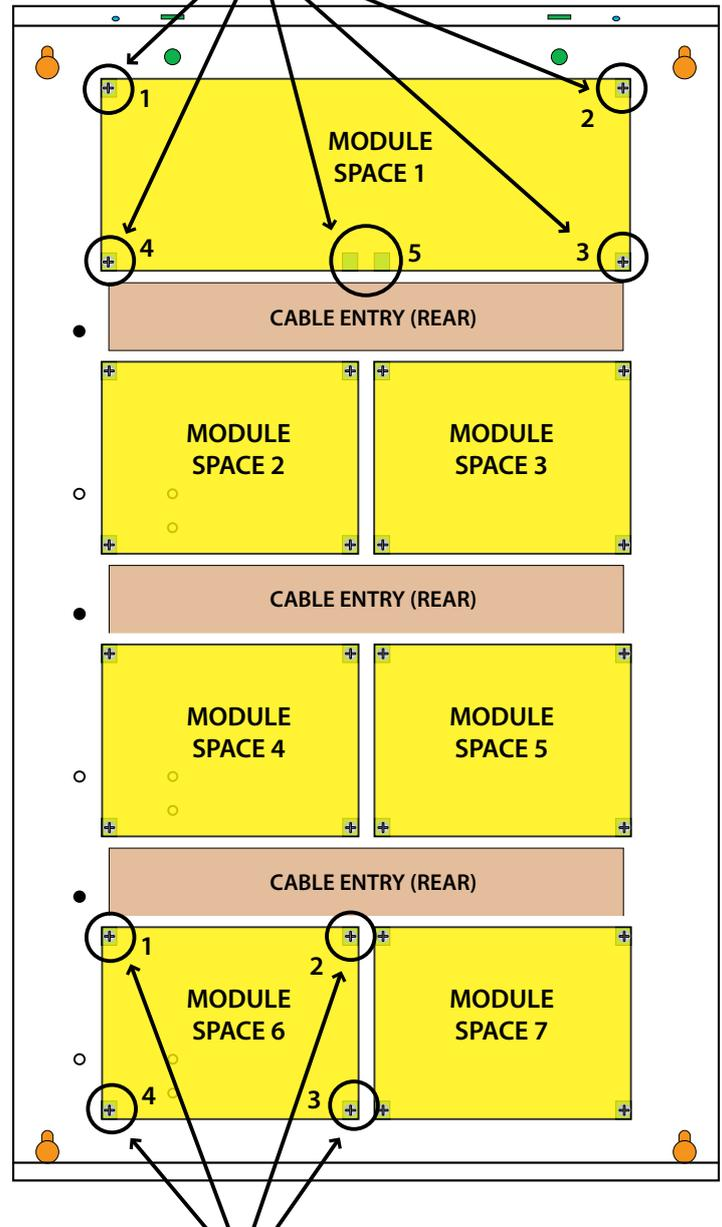
When installing small modules, you should fit 4 mounting clips as shown.
