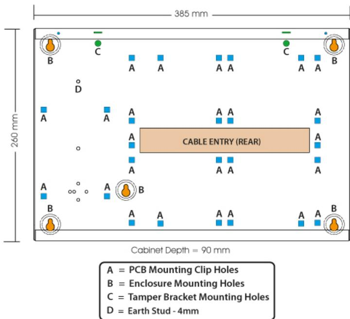
Figure 3: MW720B - Small Enclosure Details
