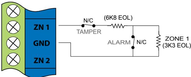
Figure 12: N/C Zone With Tamper
