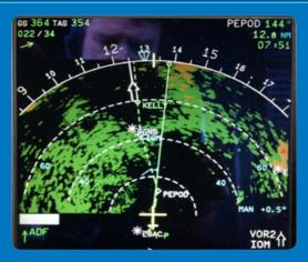
The image above is an example of the pilot's radar display and at the bottom is a cross which represents the pilot's aircraft.
