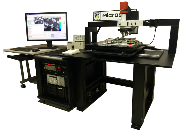
Figure 1: The SanjSCOPE™ Thermal Imaging System for back-side analysis incorporates an InGaAs sensor to cover the NIR band.
