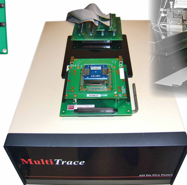
950-096 Fixture Mounted on a 950-384 Connector Motherboard
