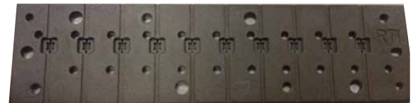
Cartridge (C) awaiting DUT loading. Airflow channels visible.
