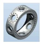
**User Controlled XYZ Positioning Sample Mount:** Integrated on top of nanopositioner stack. Includes closed-loop heater and thermometer (Cernox) control. Thermally decoupled using ultra-high thermal conductivity flexible thermal link for quick temperature changes and low position drift between 4-350K. Adds about 0.25K to base temperature.
