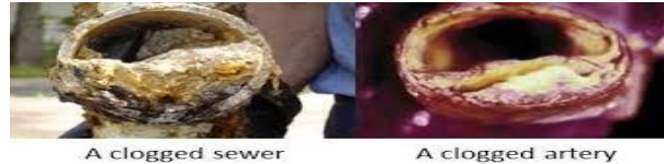
A clogged sewer
