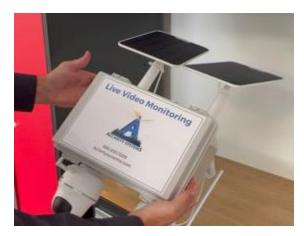
7. Turn the box over and install the mounting hardware. If you are planning on using the pole mount, use the two metal mounting tabs seen to the right of the box.
