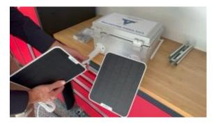
5. Route the cables down the back of the box and plug the power cables into the cameras.
