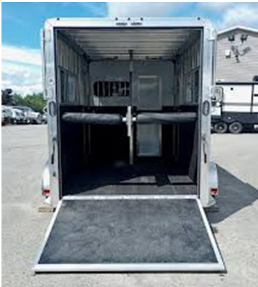
A step-up trailer. This image shows a divider inside.
