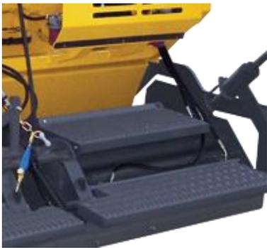
Full-floating, adjustable and vibratory screeds are standard. The 8' (2.4m) length and 13' (3.9m) width provide a solid foundation for smooth mats. The 1648 utilizes a fully heated wear plate.
