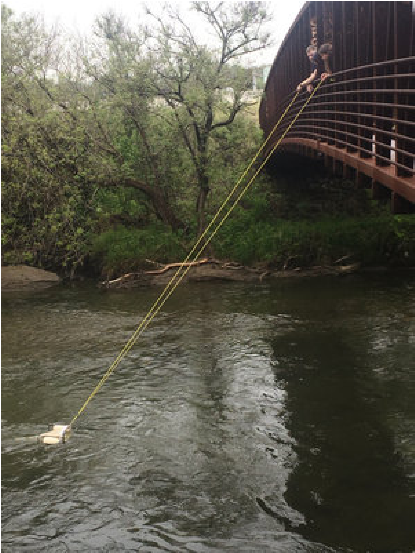
Rochman's scientific team drops a net into a stream in Toronto to collect tiny floating pieces of plastic.
