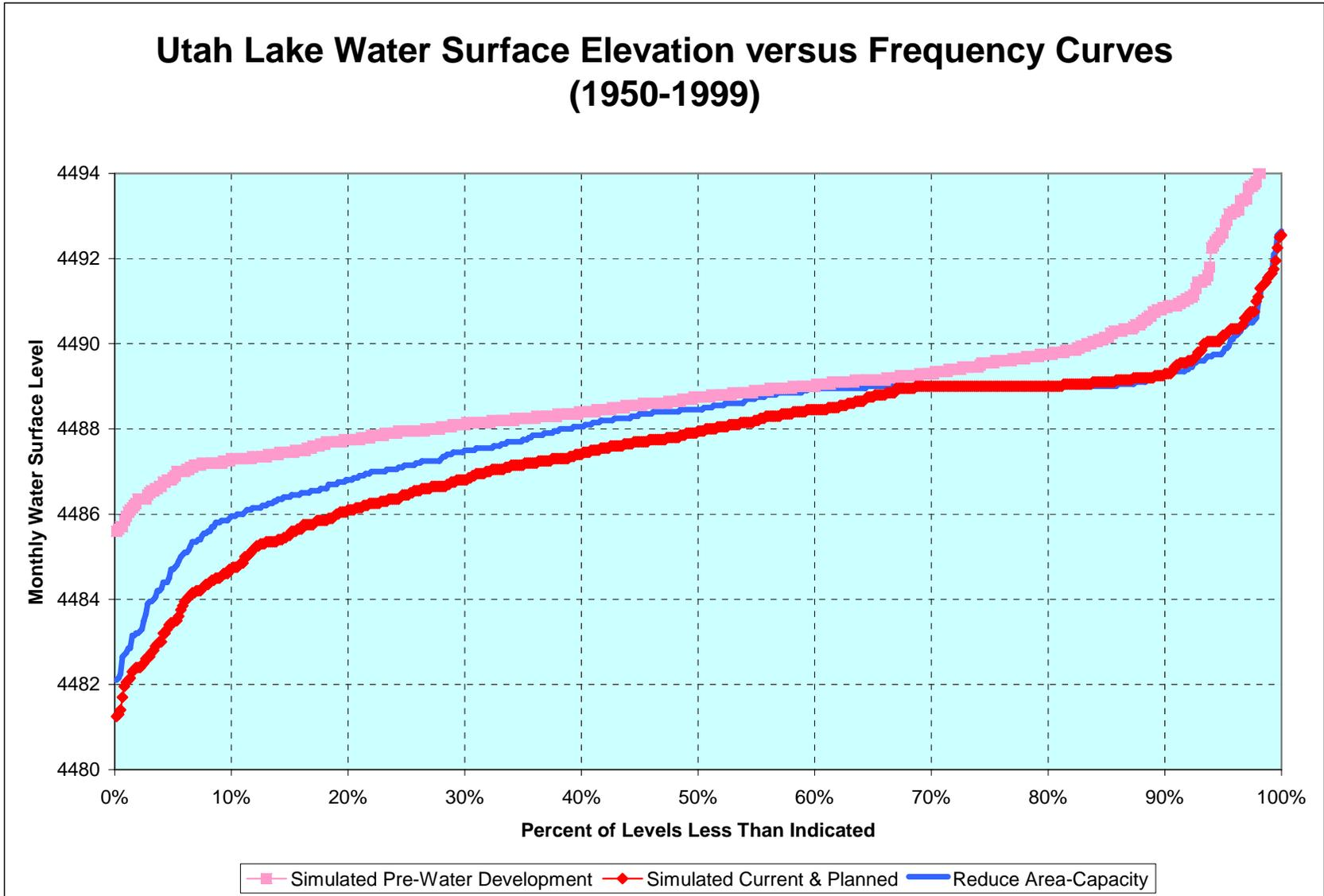
Figure 22 Simulated Utah Lake Water Levels with 50,000 Acre-feet Additional Upstream Exchange
