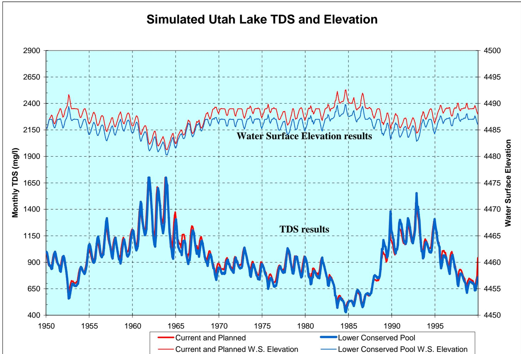
**Figure 31 Reduced Area Capacity and Current and Planned Utah Lake TDS Concentrations**
