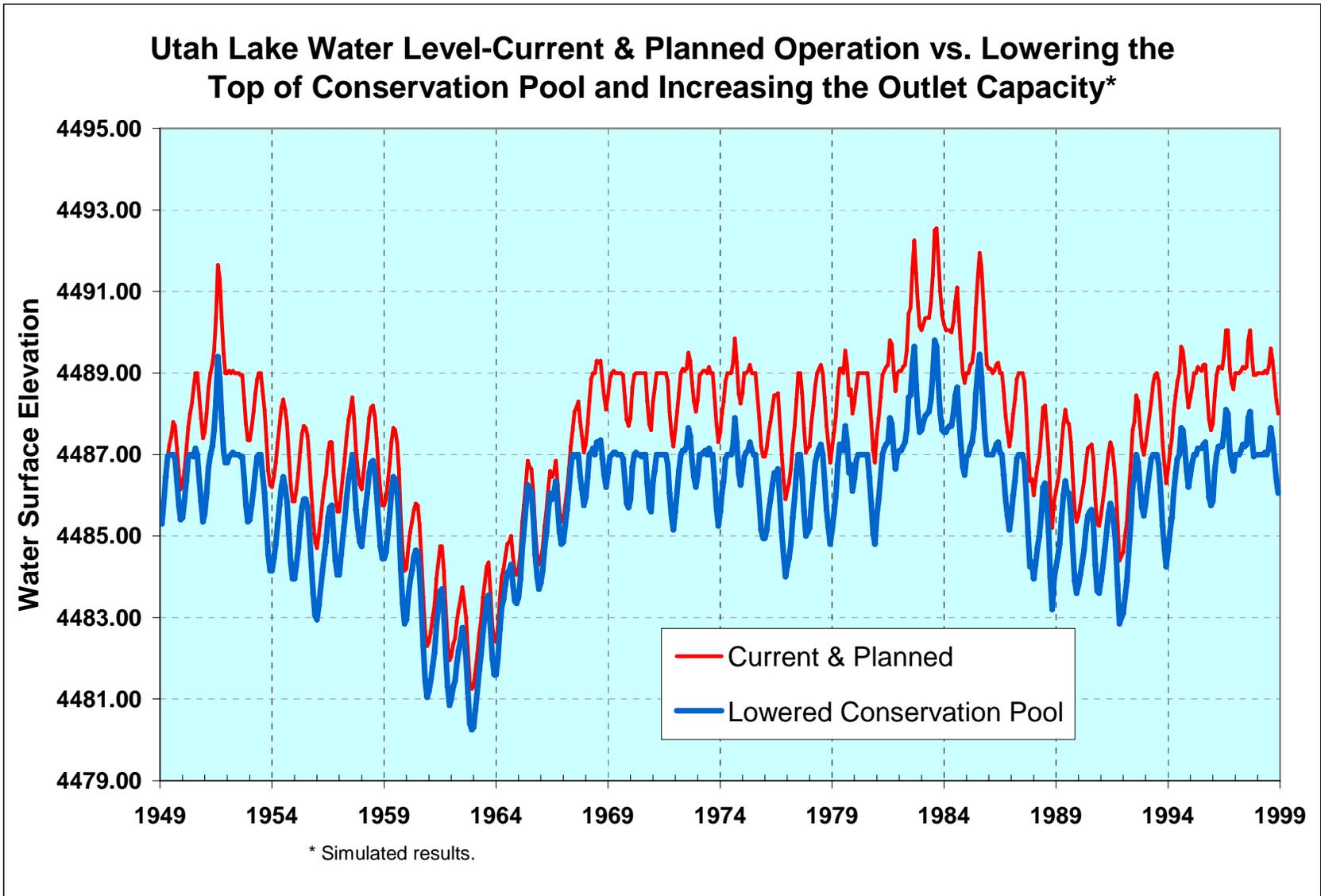
Figure 19 Simulated Water Level versus Frequency with Lowered Conservation Pool
