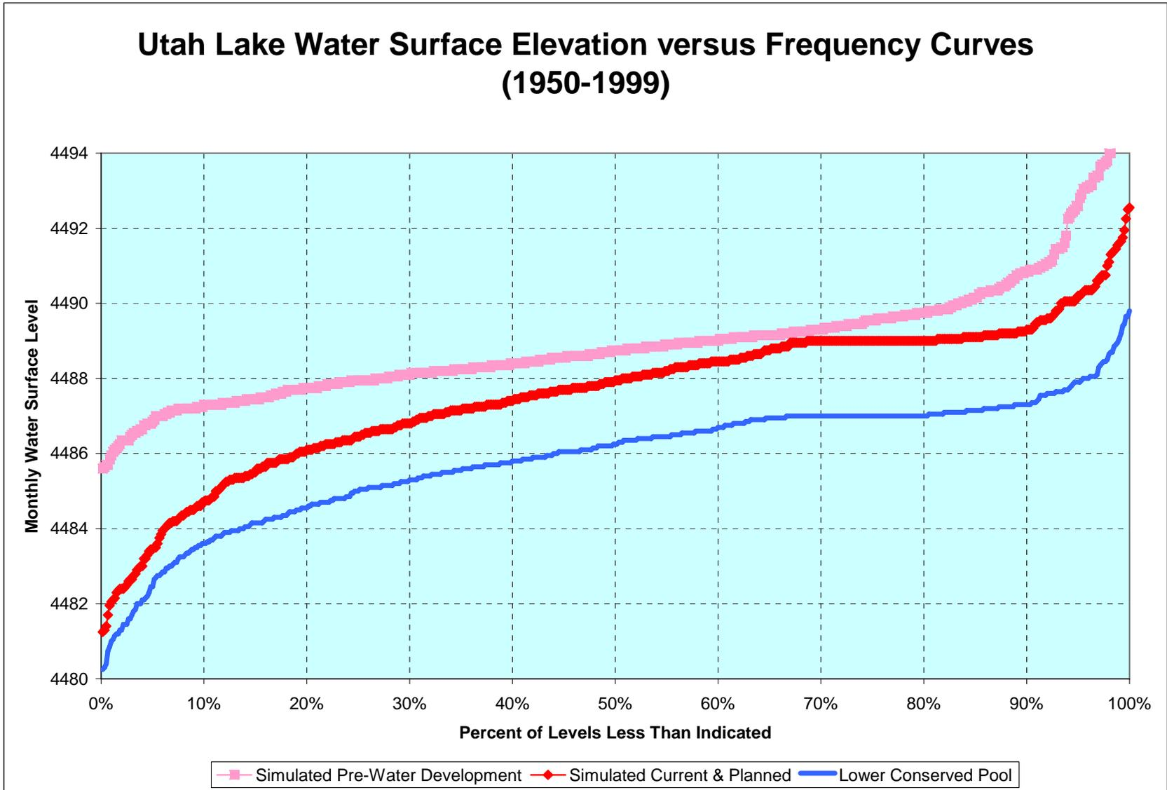
Figure 20 Simulated Utah Lake Water Levels with Reduced Area-Capacity Curve
