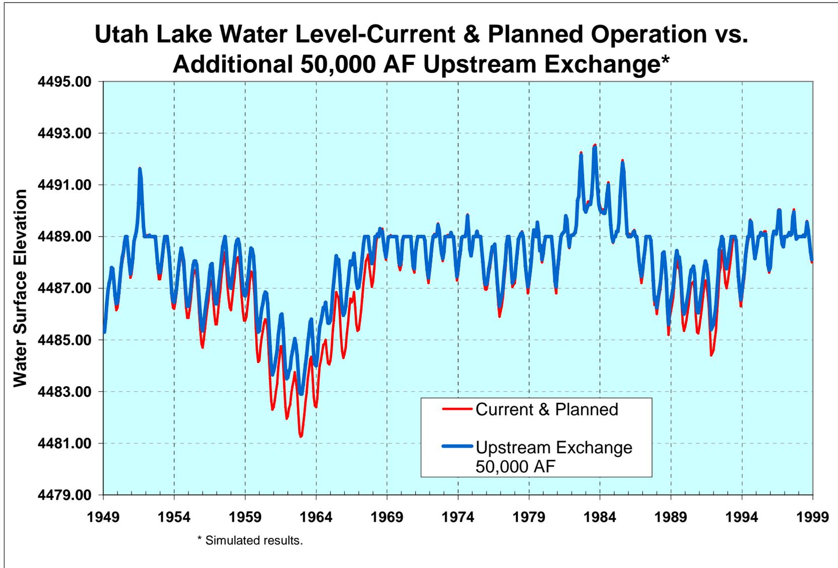
Figure 23 Simulated Water Level versus Frequency Curves with 50,000 Acre-feet Upstream Exchange
