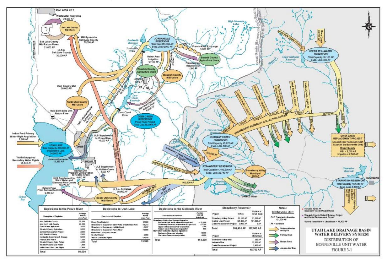
Figure 3 Utah Lake's Role in the Operation of the CUP Bonneville Unit
