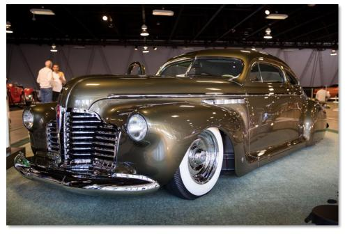
Built by Lucky 7 Customs in Antioch, California, and owned by Clifford Mattis, Dillinger wears a chopped and channeled prewar Buick body, though power comes from a small block Chevy V-8 (wearing, oddly enough, vintage Oldsmobile valve covers) instead of the original Buick Fireball 8 straight-eight. Sunday wasn't Dillinger's first time in the spotlight, either; at last month's Grand National Roadster Show, Mattis' Buick took home the 2018 Steve's Auto Restorations Award.
