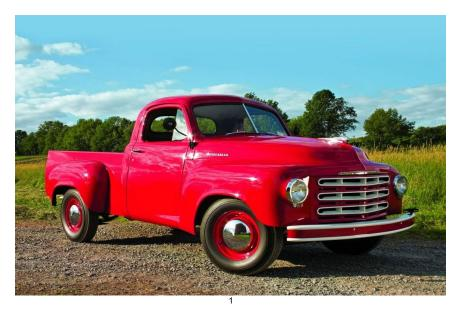
Studebaker couldn't afford to stamp out unique body panels as prodigiously as Ford and GM, so it further economized on the M5 by making the truck's fenders interchangeable from front to rear (on each side). The running boards, too, were designed to be a direct swap from side to side. Interior appointments in the M5 were sparse, in typical pre and postwar work-truck fashion. A bench seat with a rubber floor mat and a basic gauge package–viewed through a beefy two-spoke wheel–greeted drivers.
