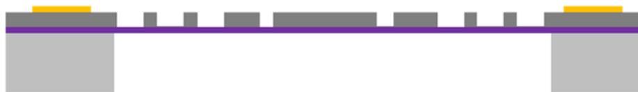
Mask #3 - Trench Backside Etching
