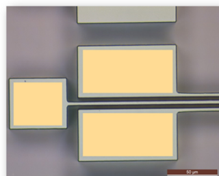
Fig. Contact PAD (yellow in color) onto the device.
