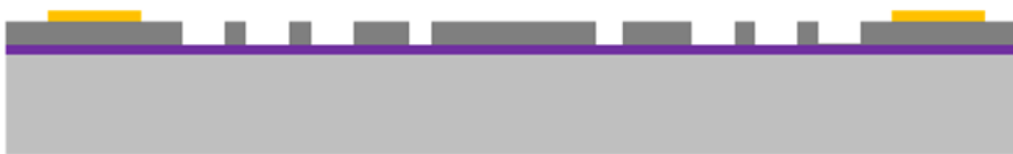
Mask #2 - Device Layer SOI
