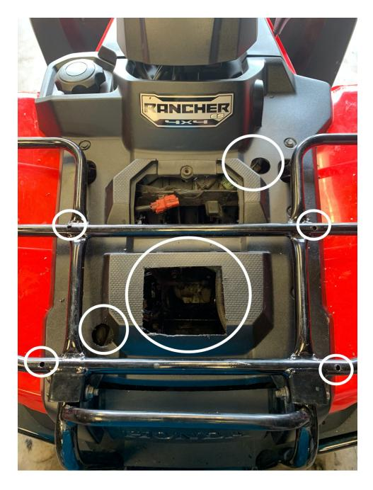
10. Drill holes in plastic and metal rack. Drill hole in plastic door as shown for fan motor wires. You do not
