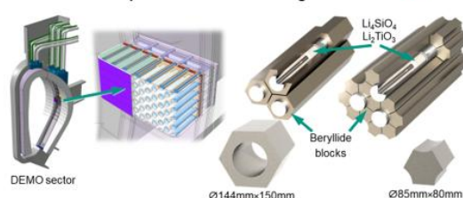
Helium-cooled pebble bed blanket design of DEMO
