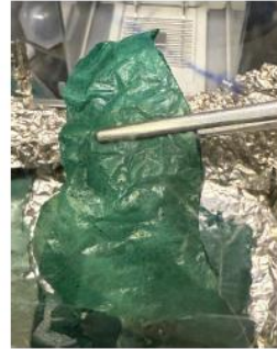
Solidified Salt surface touching on wall of Ni200 crucible
