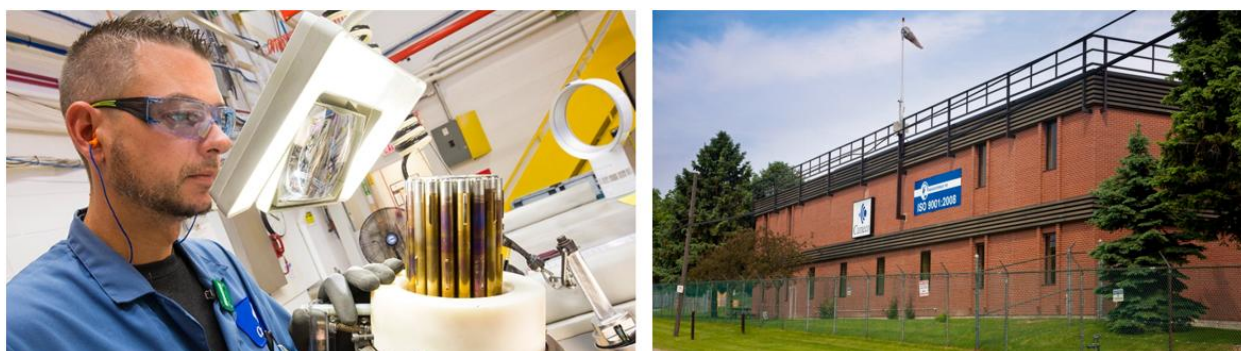
Day 2 of the 2025 Spring Meeting included tours of the Cameco Fuel Manufacturing facilities in Cobourg and Port Hope. Left: A Cameco worker assembling a zirconium alloy fuel bundle, which is brazed together using beryllium. Right: An exterior photo of Cameco's Port Hope facility. Both photos courtesy of Cameco Fuel Manufacturing.
