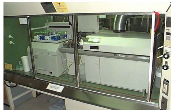
(ICP-MS installed at SRNL radiological lab)
