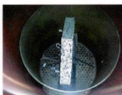
HIPed Blank inside protective cover
