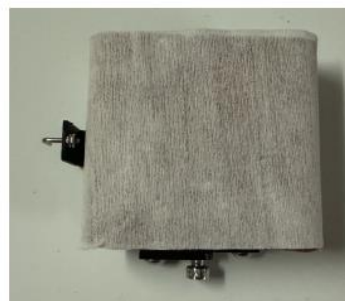
Fig 3. Clean weighed wipe attached to cart
