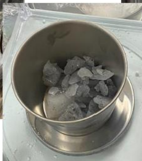
Solid beryllium fluoride for making FLiBe in the lab.
