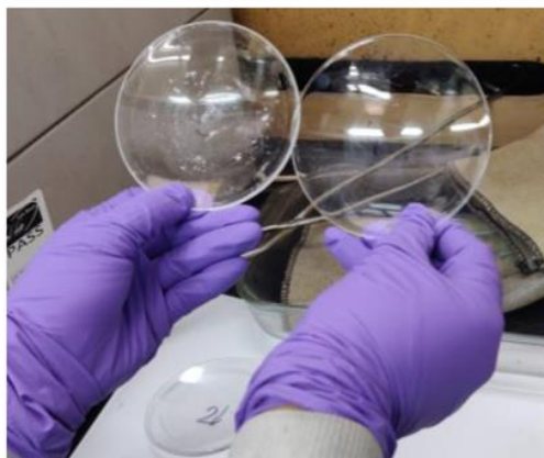
Glass plates spiked with beryllium-containing solution in known amounts were used in the previous study [6]
