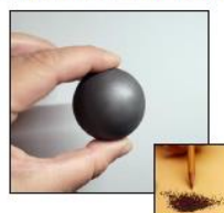
Liquid Fluoride Salt Coolant Flibe (2LiF-BeF 2 )
