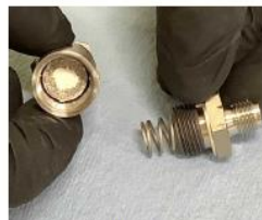
Flibe "snow" accumulated in off-gas lines
