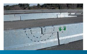
The modular BarrierGuard 800 Opening Gate is assembled with standard sections, with wheelunits mounted inside. The outer ends that connect to concrete barrier or guardrails are equipped with hinges. If desired a third hinge can be added in the middle for maximum use. The BarrierGuard 800 Opening Gate can be safely opened or closed in just a few minutes using only manual power.
