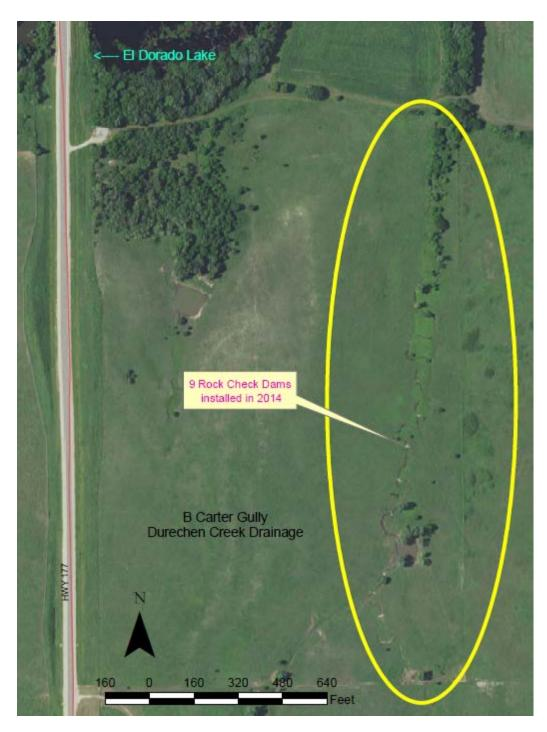
The gully surveyed in the Durechen Creek drainage area was determined by the Soil and Water Assessment Tool (SWAT) model to be in a high priority area for sediment and nutrient runoff. The soil type in the field where the gully is located is Labette-sogn silty clay loam, 0-8% slope. This field is burned on a regular basis (every other year). Stocker cattle are put in this pasture from late April to the end of
