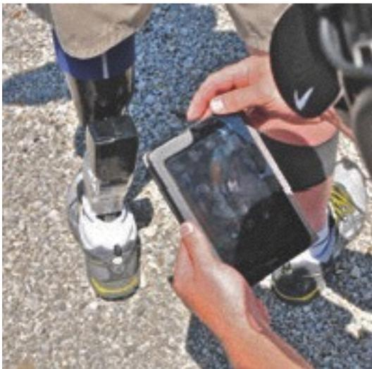
*BiOM can be adjusted on the fly via Bluetooth-enabled tablet PC. This allows the foot's sensors to be tailored to the wearer's needs instead of the wearer learning to work within the confines of a preset program.*
