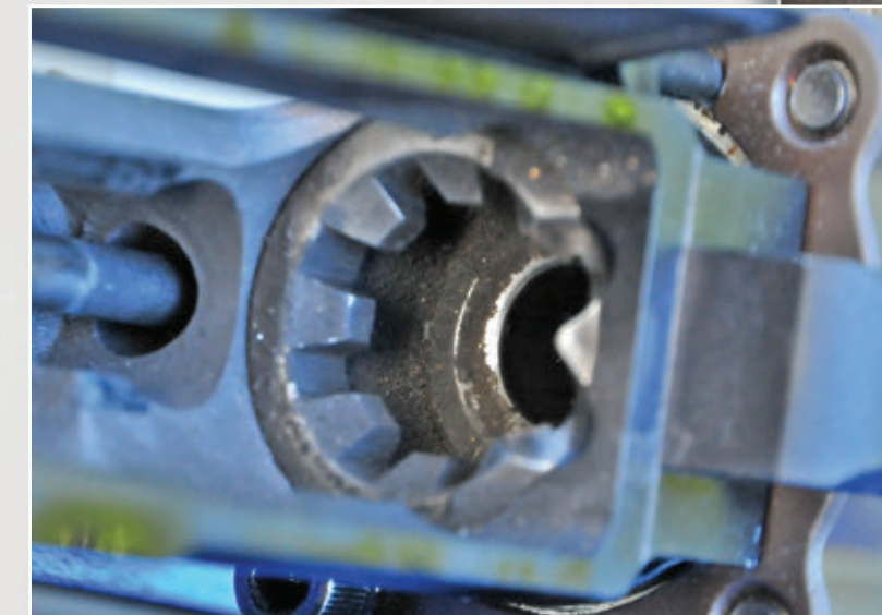
Barrel extension is filthy, and yet it's dry. A wall of carbon is pushing against the bolt face as it tries to lock into battery. Even with all this fouling, the rifle continued to run.
