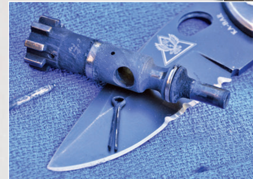
Cleaning NiB-X coated parts is as easy as scraping away the carbon with a knife edge. Little effort is needed to bring back the silver shine of NiB-X.
