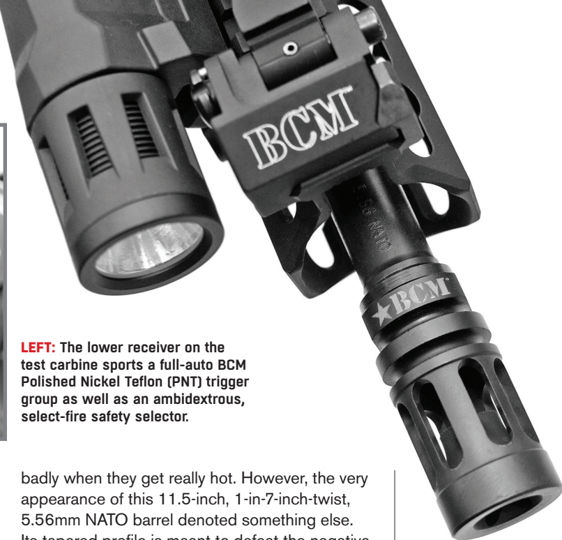
ABOVE: Even while firing full-auto bursts, the BCM Gunfighter Mod 0 compensator helped reduce recoil and muzzle rise for quick tracking between targets.
