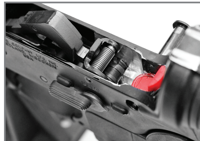
LEFT: The lower receiver on the test carbine sports a full-auto BCM Polished Nickel Teflon (PNT) trigger group as well as an ambidextrous, select-fire safety selector.
