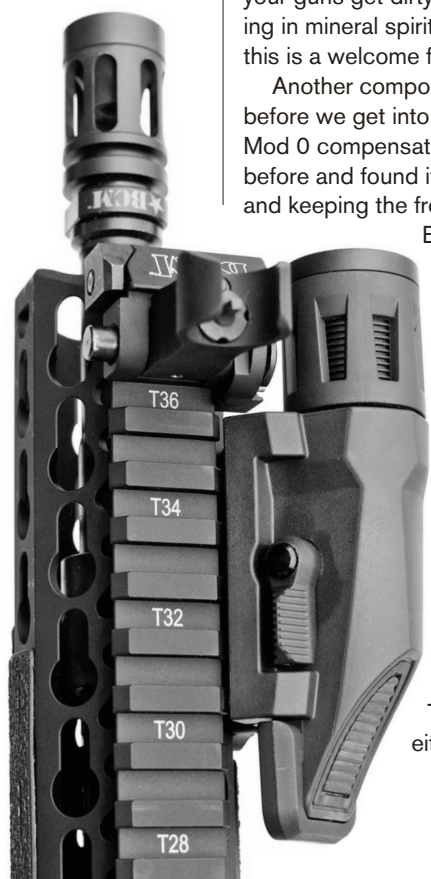
BELOW: The free-floating KMR-A handguard features T-marked slots on the top rail, and the author added flip-up sights as well as an Inforce WML light.
