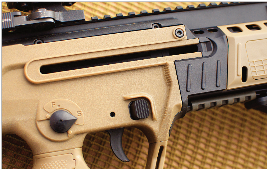
The charging handle can be switched to the left side, but you'll need a conversion kit.
