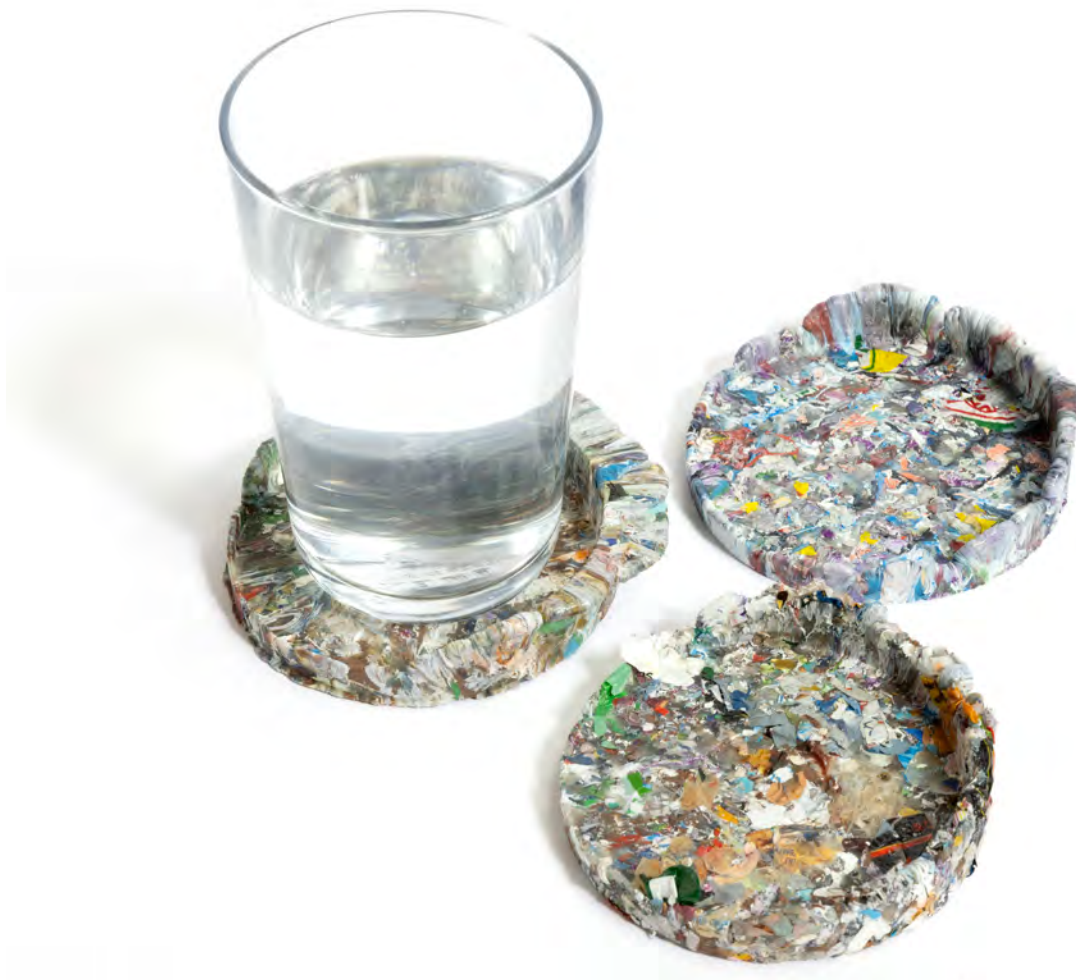
Pressed sheet and coasters made from soft plastics.
