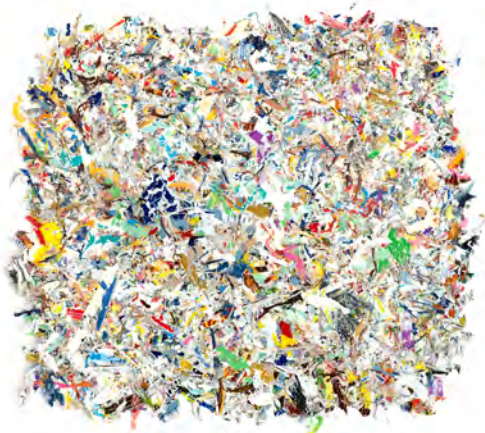
Top: Shredded snack wrappers and chip bags. Middle: Shredded materials in heat press. Bottom: Pressed sheet after heat press process.
