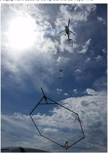
Photo 2. Airborne Electromagnetic (AEM)
