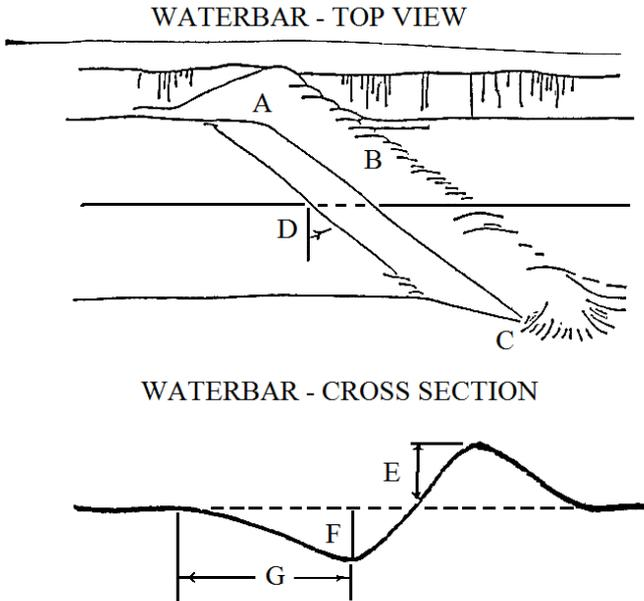
1. Specifications for *waterbar* construction on *forest roads*, trails and *firebreaks* must be site specific and should be adjusted to existing *soil* and slope conditions.
