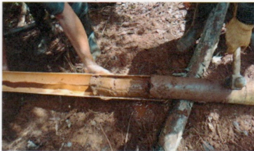
Figure 7.1.3: Recovery of drill core from core barrel
