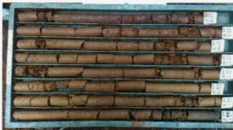
Figure 7.1.3: Recovery of drill core from core barrel
