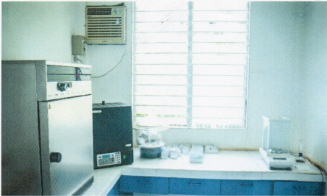
Figure 8.1.6: Electric Drying Oven
