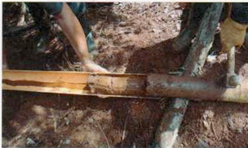
Figure 7.1.3: Recovery of drill core from core barrel
