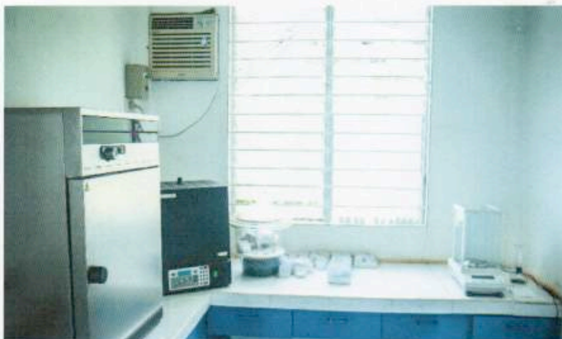
Figure 8.1.6: Electric Drying Oven
