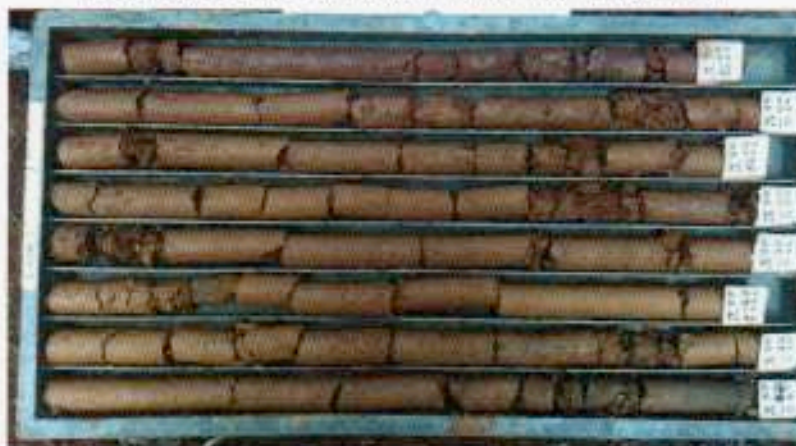
Figure 7.1.3: Recovery of drill core from core barrel
