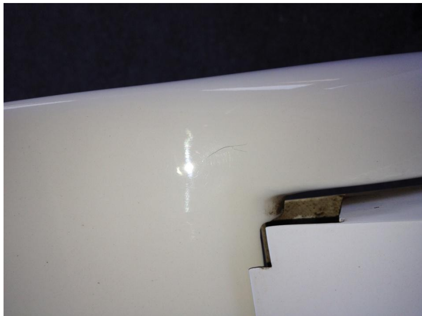
superficial crack in paintwork
