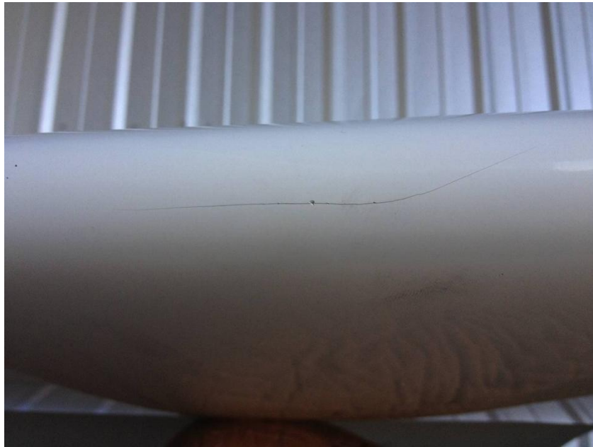
superficial crack in elevator leading edge
