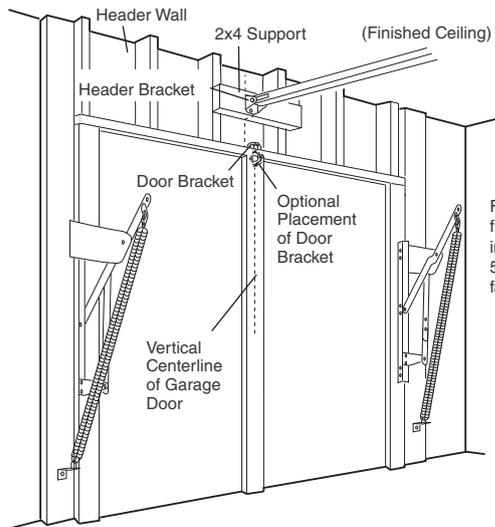
For a door with no exposed framing, or for the optional installation, use lag screws 5/16"x1-1/2" (not provided) to fasten the door bracket.
