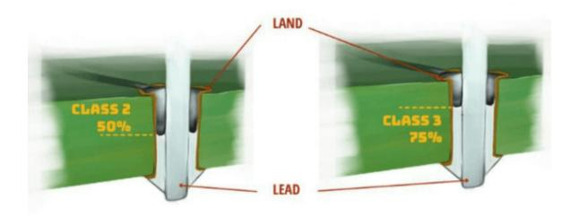
Besides, you can also find the difference in the amount of barrel fill. For Class 2, the amount to fill the barrel for a through hole is 50%. While Class 3 requires 75% of barrel fill. This is one of the delicate processes of getting the proper amount of fill or pastes into the smaller plate of through holes, so one must be very careful during this process.
