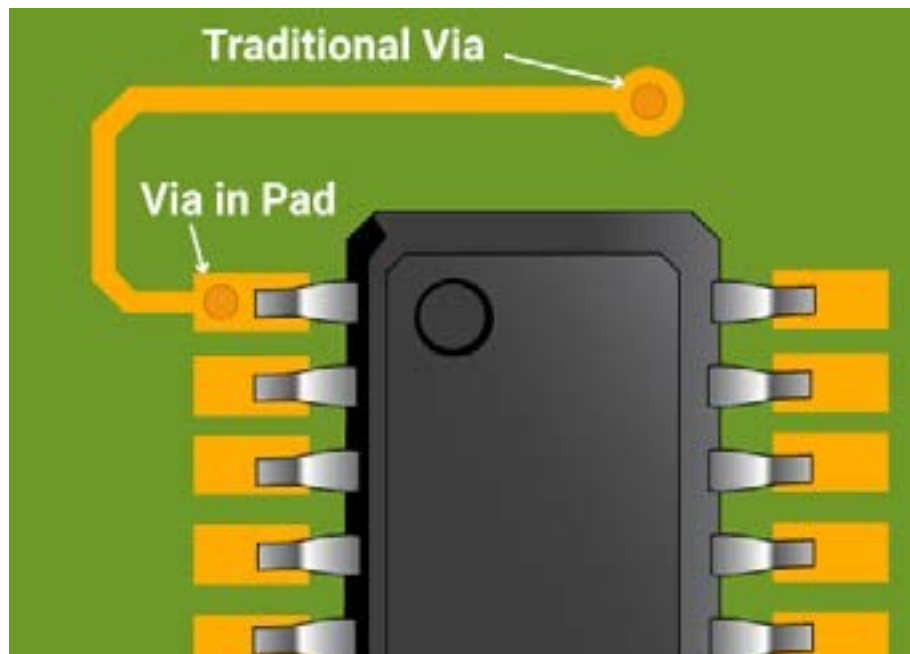
Via-in-pad Vs traditional via
