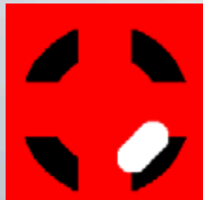
CAM snapshots showing copper slivers
