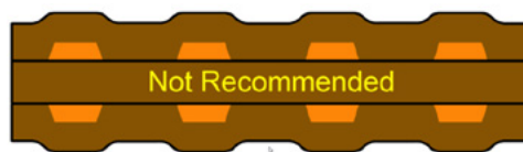
Figure 4.7 Adjacent-layer copper traces are not recommended
