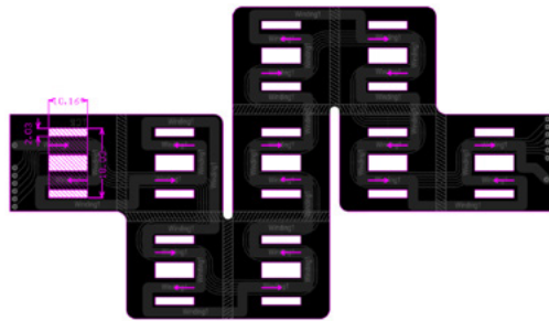
Figure 5.8 Mechanical 1 layer showing the board outline as well as winding direction arrows for guidance. The final core-and-flex assembly is shown below. Note that this could be integrated within a rigid-flex design where the majority of the circuit is on a rigid 2-layer PCB, with the flex part being used to get the additional layers needed for all the core windings. Of course, there is going to be a cost trade-off between using a large flex area versus just adding heaps of layers to a rigid-only design.
