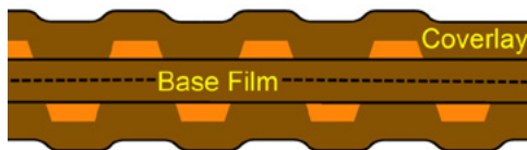
Figure 4.8 Staggered adjacent-layer traces are preferred
