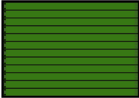
Figure 5.12 The Same panel size - the folded flex design doubles the per-panel output yield
