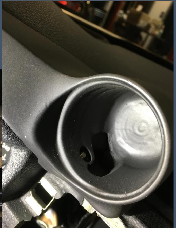
Then trim out a small piece of the backing to allow for clearance of your wires
