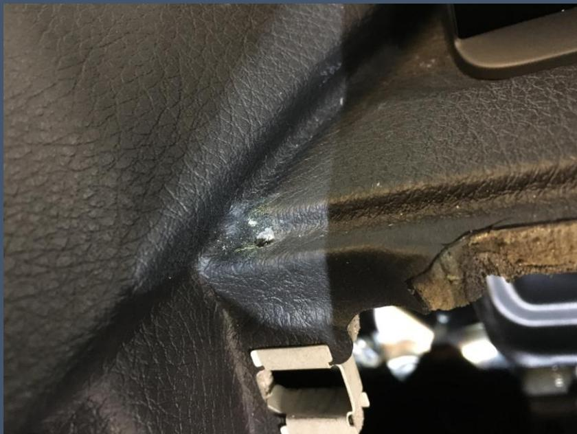
Set your screw/stud depth. It is important that the depth is set accurately to make the nut flush when tightened in the pod later. Temporarily mount the pod to make sure the depth is perfect.
