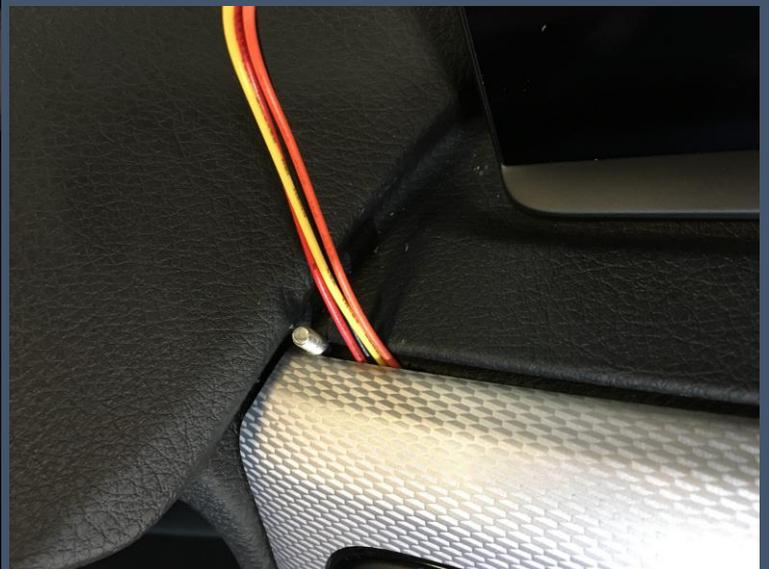
Now proceed to feed your wiring through the gauge pod bottom hole allowing yourself to plug the gauge in later, slide your gauge pod down over the stud as shown
