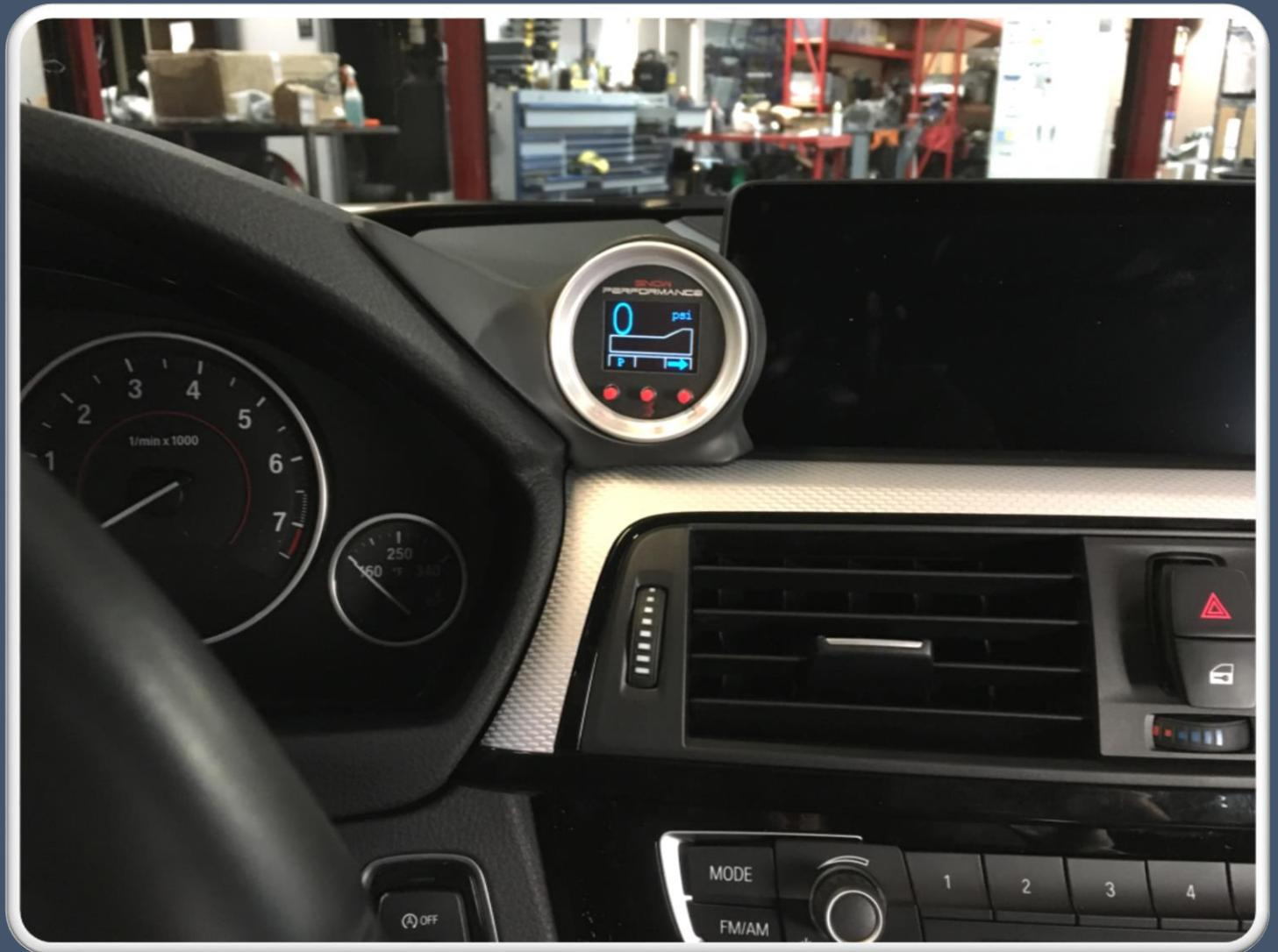
In the case of a snow performance gauge that has no connection in the back of the gauge you may have to be creative and run your wires through the pod and make all your connections leaving extra room to slide the pot into place
