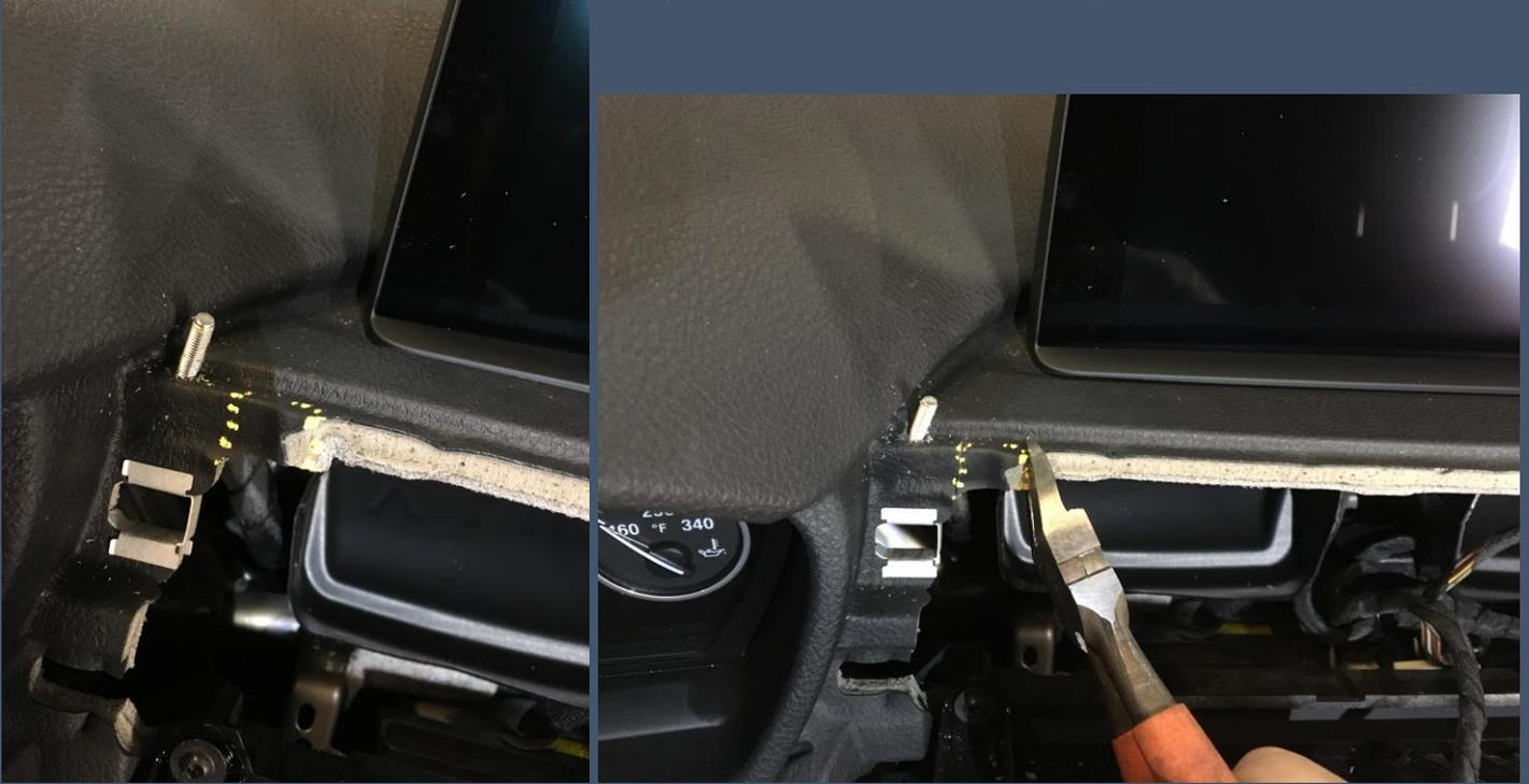
Notice that you will not cut into the visible portion of the dashboard for larger wires cut back the underlining plastic a bit farther.
