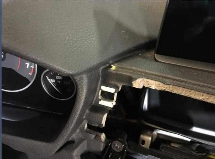
Carefully drill your hole using a 7/64 in drill bit. A slightly larger bit may be used but the hole needs to be tight enough to hold the bolt in place on its own essentially making it in to a stud.
