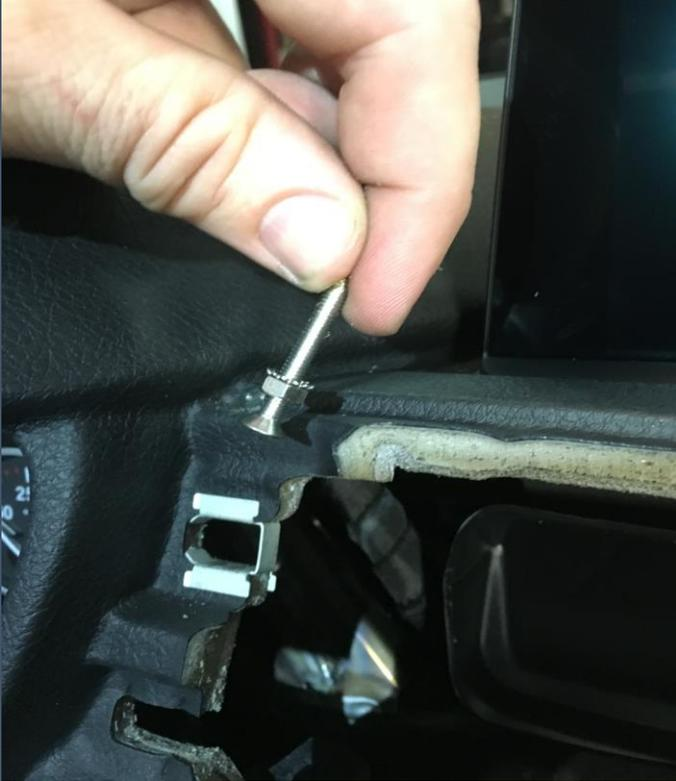
Insert your screw through the hole from the backside
