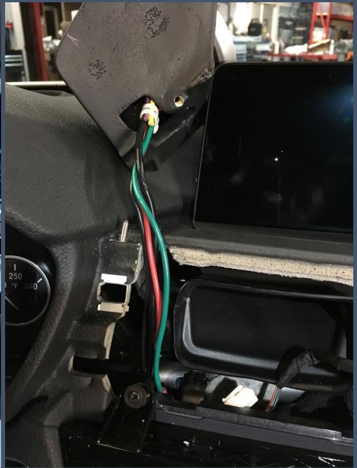
Once the pod is tighten down and fully mounted, you can then pull the wires through the dash from underneath like so.
