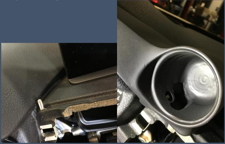
Then trim out a small piece of the backing to allow for clearance of your wires
