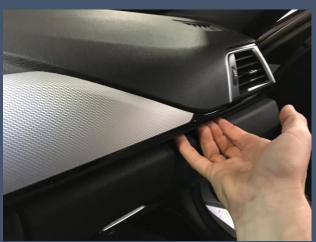
Then unplug the two connectors on the back of the center vents to remove the panel complealy
