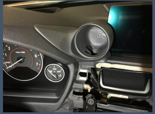
Use a piece of wire bent at 90°, a pic or even the provided screw To Mark your hole location. That will be drilled shortly, as it needs to be in the perfect location.
