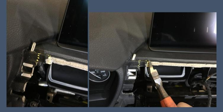
Notice that you will not cut into the visible portion of the dashboard for larger wires cut back the underlining plastic a bit farther.
