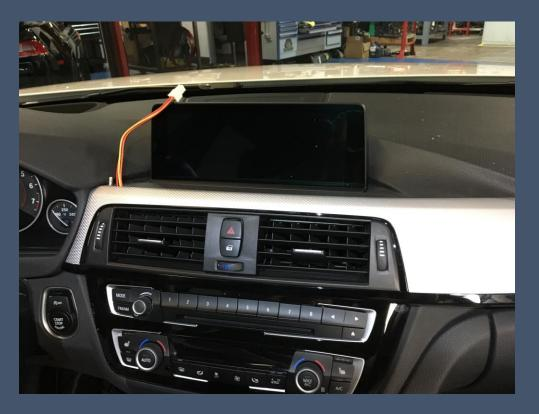
You will notice that the bezel from the front will look fully seated but in fact if you drilled your Stud hole correctly you will see that it keeps a very small gap as to give gauges with heaver wiring a little more room. The pod itself is designed to fit this additional gap perfectly.
