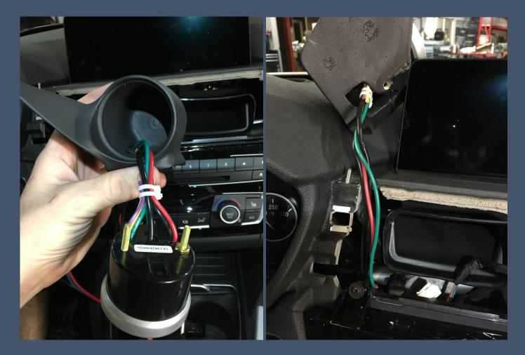
Once the pod is tighten down and fully mounted, you can then pull the wires through the dash from underneath like so.
