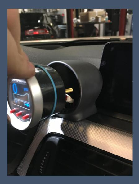
This is where the need of a rubber band or grommet will be helpful to ensure a tight fit into the pod opening.
