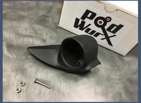
Then start by just putting your new Podwurx pod on to the dash in its future location just to make sure your pod fits the natural contours of your dashboard. Then remove the center trim popping each clip gently all the way across as to not crack the plastic
