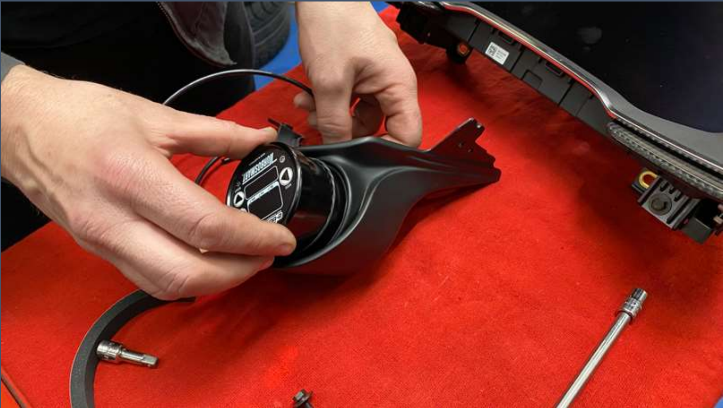
Next slide the gauge in to the pod making sure the rings slide in to the pod smoothly
