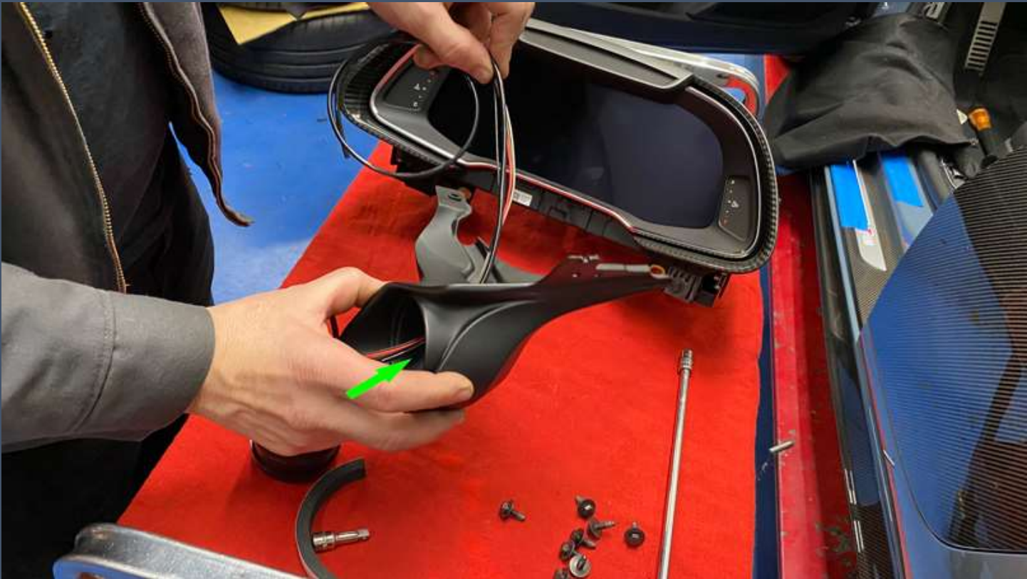
Pass the gauges wiring though the pods passage way.
